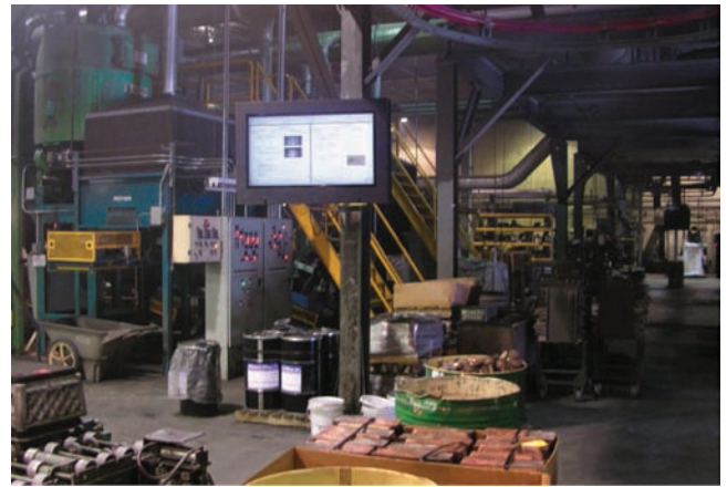
Figure 2-53 HMI installed in an industrial environment. Source: Photo Courtesy PC Enclosures, http://www.pcclosures.net .
