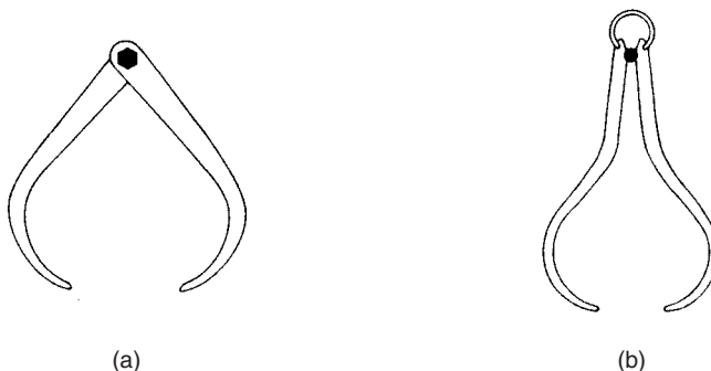
Fig. 21.3 (a) Standard calliper; (b) spring-loaded calliper.
