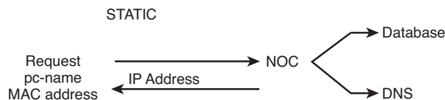
FIGURE 5-12 Manually updating the A record
