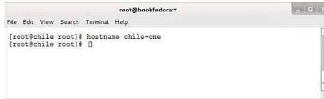
FIGURE 9-55 An example of using the hostname command to change the name of the Linux machine
