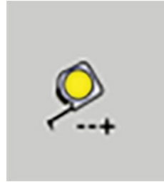
Figure 4-23: The - - + signs mean the Tape Measure is in measure and guideline mode.
