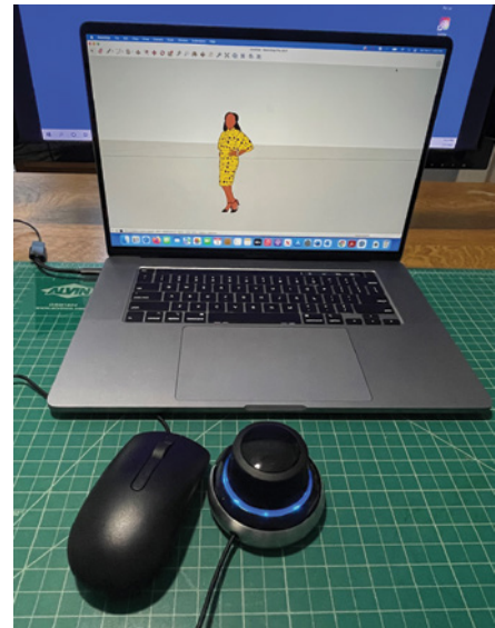
Figure 2-3: The 3D mouse is used with a traditional mouse.
