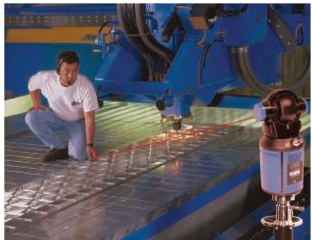
This laser tracking device, by Faro Technologies, enables quality control personnel to measure and inspect parts and tools during production. The portable tracker can measure objects from 262 feet away and takes up to 1,000 accurate readings per second.
