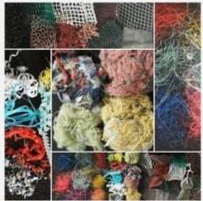
Figure 3 ECONYL® nylon yarn is not only 100% regenerated, it is also regenerable. These discarded fishing nets, fluff (upper part of the carpet) and plastic components will be transformed into nylon for carpets, having the same quality as virgin nylon. When the carpets reach the end of their lifecycle, the fluff can be regenerated back into new fibre, without any loss of quality.
